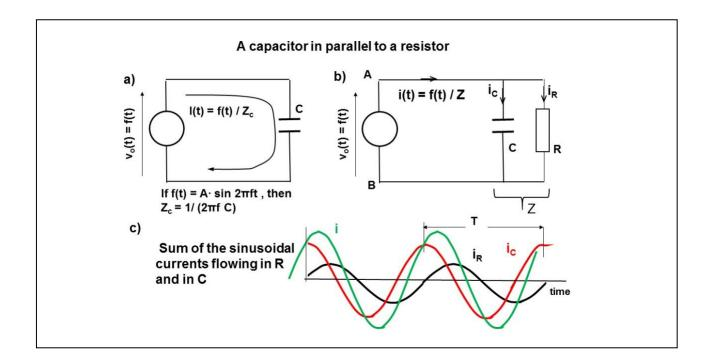
Fig. 2. Capacitive loads. a) circuit including a generic generator and a capacitive load, b) circuit with a load including a resistor and a capacitor in parallel: i = iR + ic, c) plot of the sinusoidal currents i, iR, and ic, when vAB is a sinusoidal voltage, that is  $f(t) = vAB(t) = v_0(t) = A \cdot sin(2\pi ft)$ . Note that the peak value of i is not the sum of the peak values of iR and ic. Also note that R is not affected by frequency but  $Z_c$  is.
