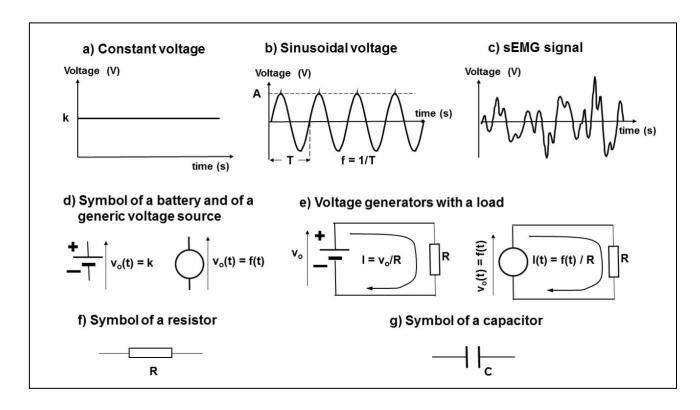
Fig. 1. a) constant (or DC) voltage, such as that produced by a battery, b) sinusoidal voltage, such as that of the power line, c) general waveform, such as that of sEMG, d) symbols of a battery and of a generic generator, e) battery and generic generator connected to a resistors, f) and g) symbols used to indicate a resistor and a capacitor.
