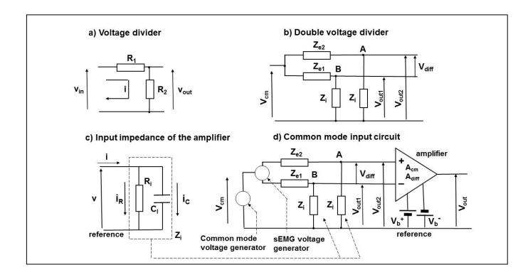
*Fig. 3.* Voltage divider. a) concept of voltage divider made of two resistors, b) double voltage divider with impedances, c) input impedance of a bioelectric signal amplifier, d) circuit for the analysis of the common mode voltage present at the input of a bioelectric signal amplifier.
