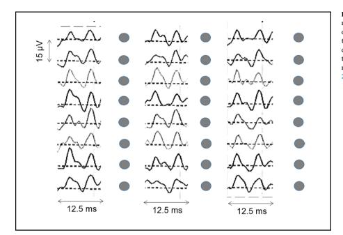
**Fig. 4.** Example of highly correlated noise across the monopolar channels of an 8x3 electrode grid applied on a piece of pig skin to avoid any sEMG contribution. This noise is reduced but not cancelled by the differential detection. Interelectrode distance = 10 mm in both directions, electrode diameter = 3 mm. Modified from (Russo and Merletti, 2017).
